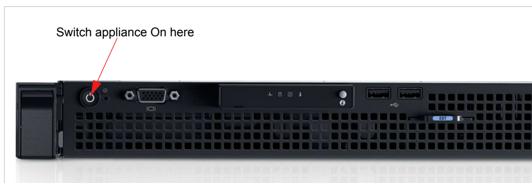
Figure 2-10 Power Switch - Base System Appliance
